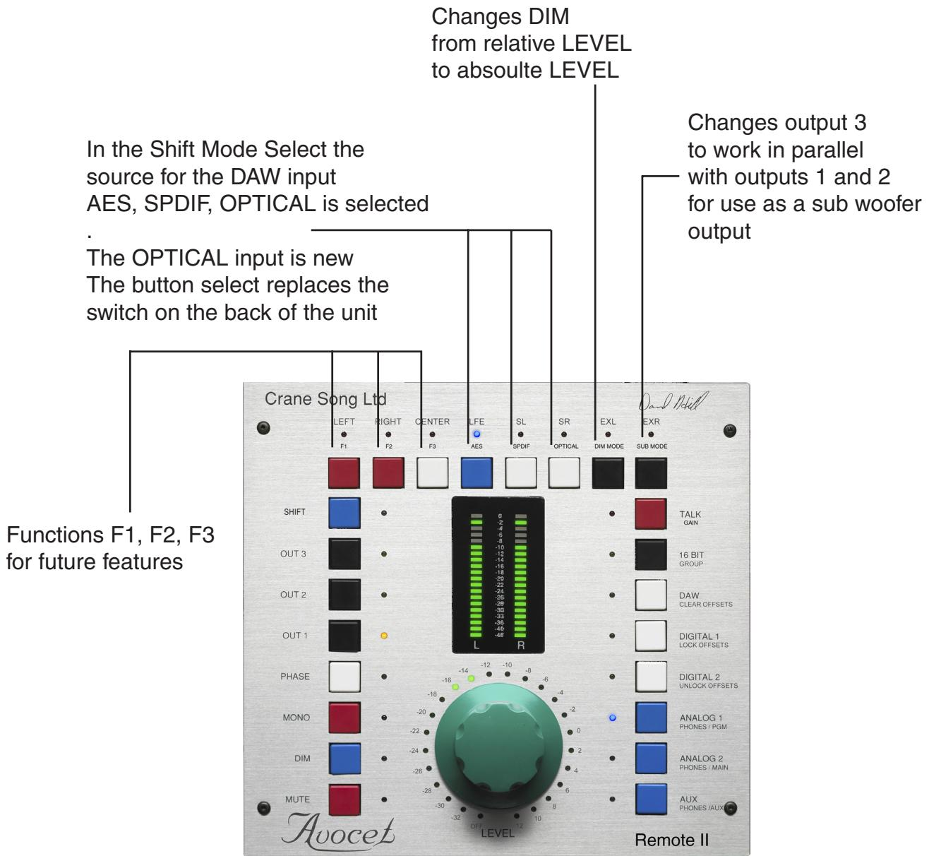
Note: The addition of selectable digital inputs in the shift mode requires the selection enabled D/A converter, which ships will all current production units
