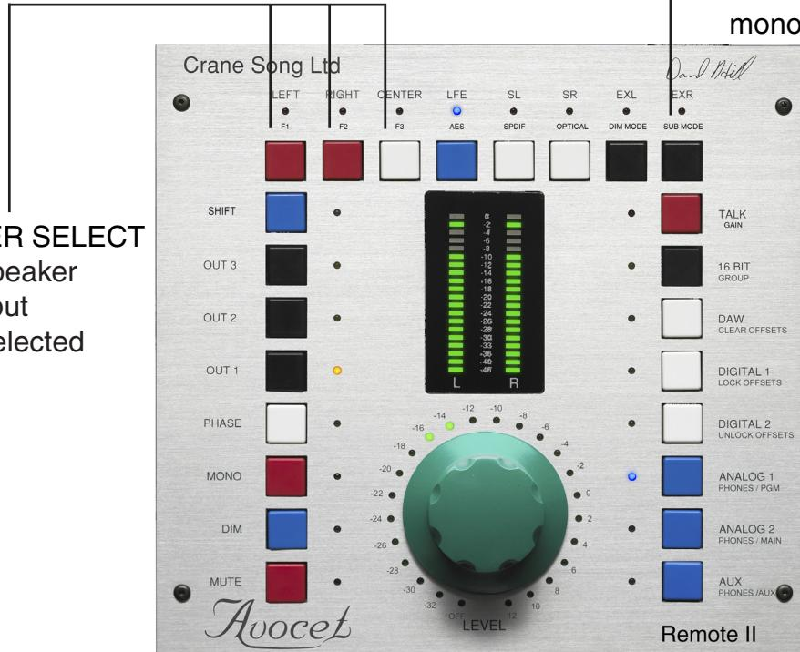
In OUT 1 SETUP SELECT turning this button on will cause the unit to be in surround mode at all times (Transparent Surround Mode) the mono speaker select function determines the active speakers when mono is selected
