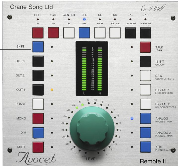
When holding down a button for gain trim; or speaker setup, the led now provides feedback that the button was held for the required time. The led will wink out for 1/2 second and then come back on. In the previous version there was no feedback to the user on mode change. This applies to the 6 input select buttons, the mono button, and the speaker buttons for selecting the mono output channel.
